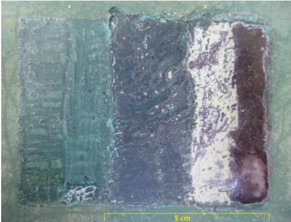
Figure 4. Investigative cleaning section revealing 3 layers of green paint and a white primer.
