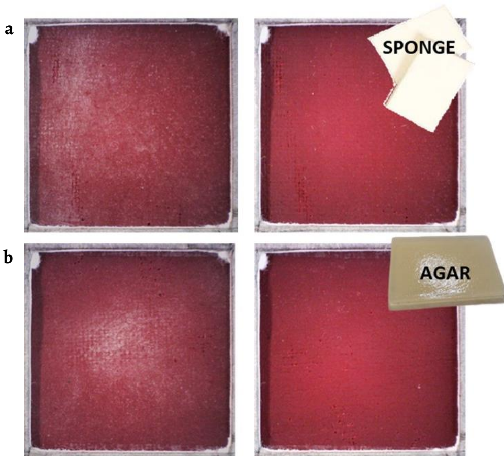
Figure 7. More deteriorated TPU-coated fabric with blooming, before (left) and after (right) cleaning with the best identified wet cleaning methods: a ) sponge/water and b ) agar-agar gel.
