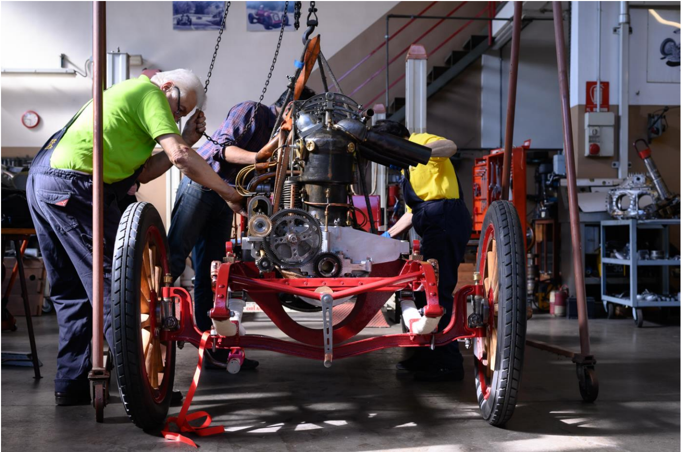
Figure 10. The positioning of the engine on the chassis.
