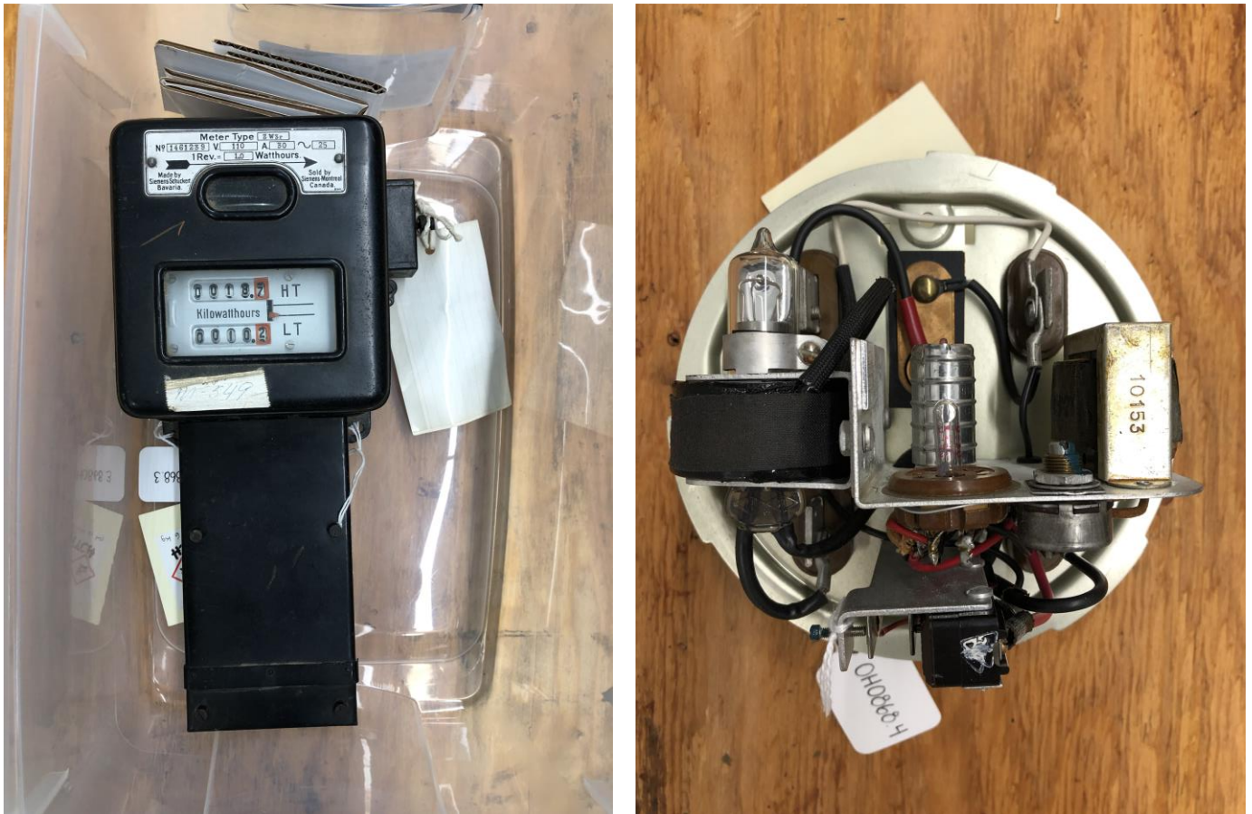
Figure 8. Examples of mercury switches in electrical meters: a) Siemens meter; b) Lumatrol meter.
