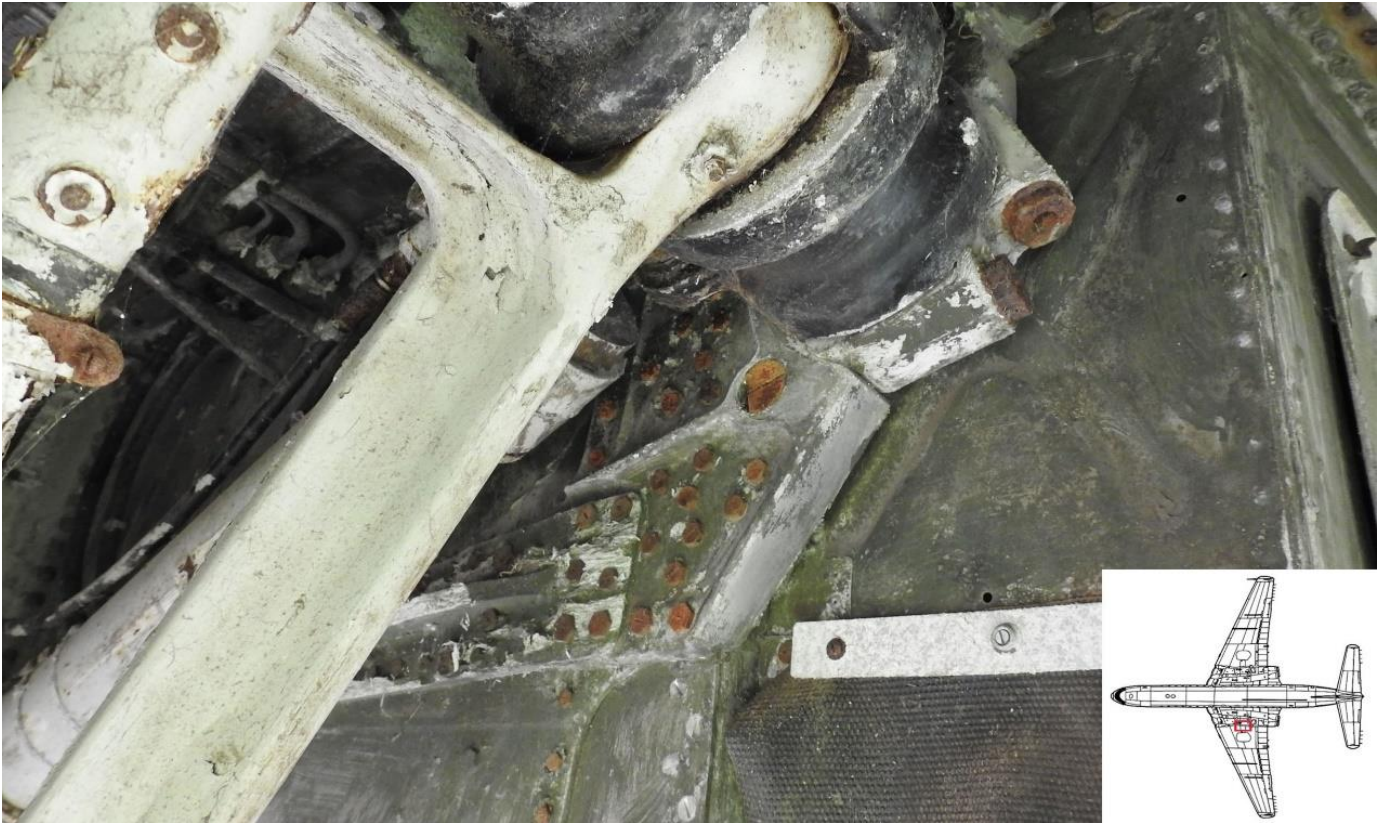
Figure 3. Corroded main undercarriage attachment point.
