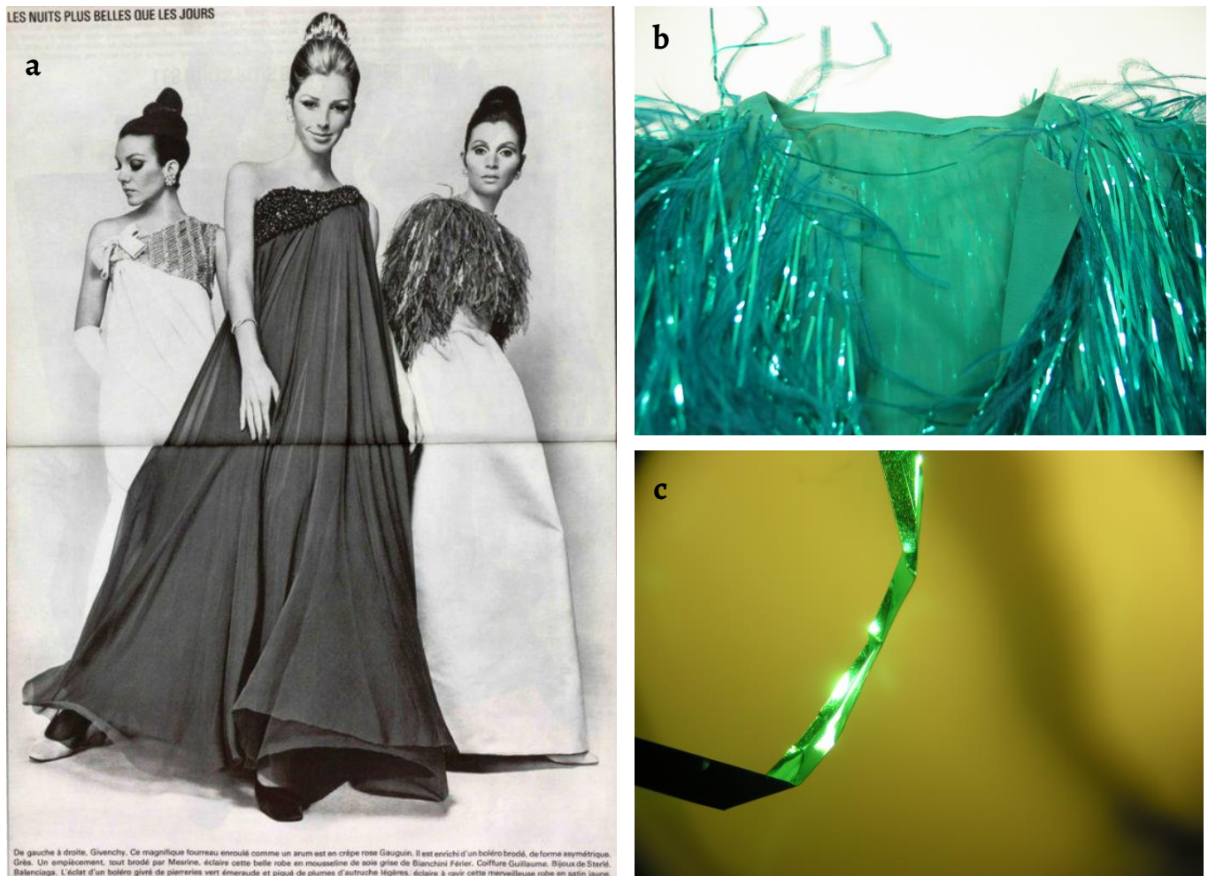
Figure 17. PET plastics used in fashion: a) Balenciaga's Bolero jacket advertised in 1966 ( L'officiel de la mode n°537: 118-119); b) Balenciaga, Cristobal, Night Bolero with PET plastic strips and turquoise feathers, Balenciaga-Eisa, 1966, Cristobal Balenciaga Museum; c) Usual twisted "neck" deterioration present in PET strip simulating Lurex.
