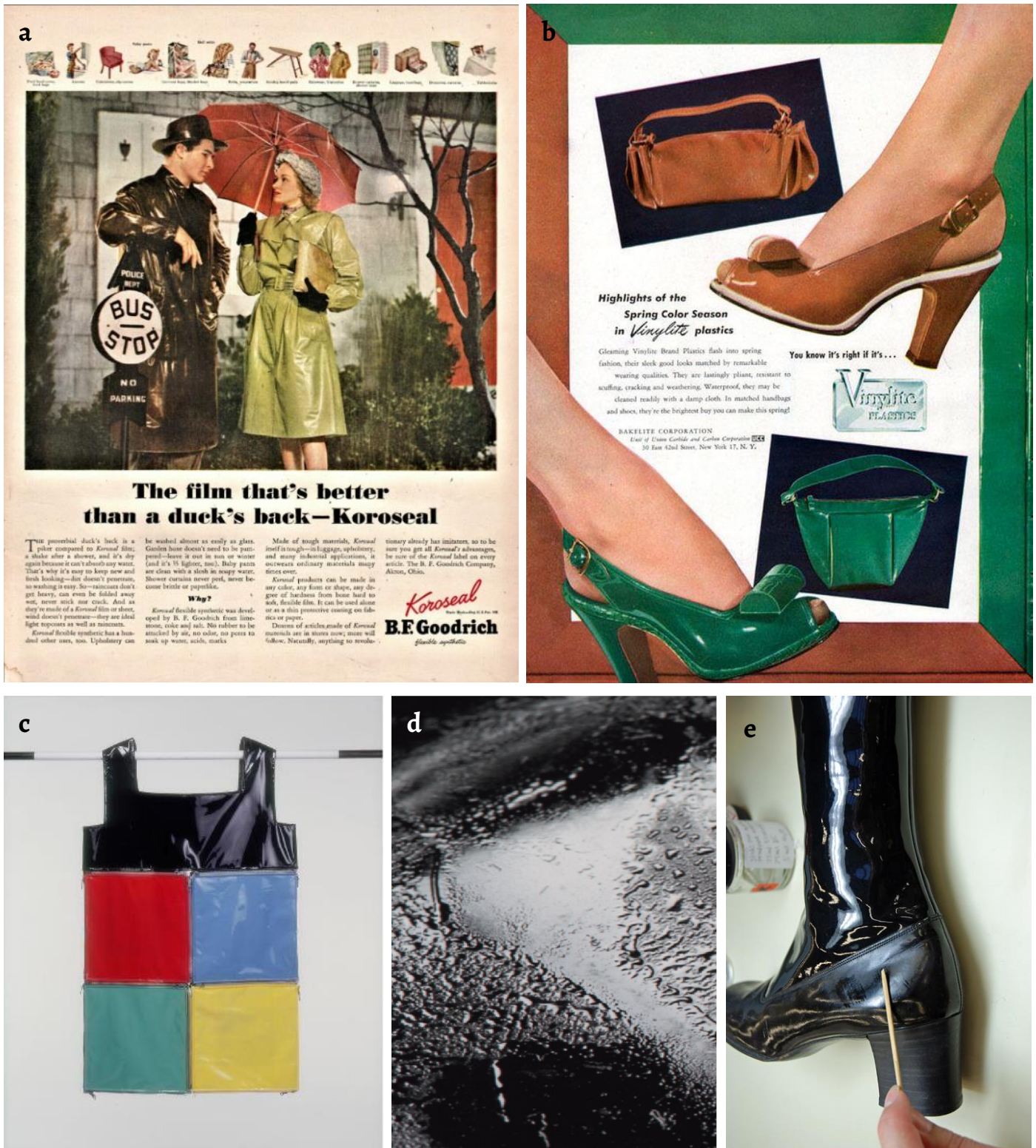
Figure 14. Advertisements of PVC costumes: a) B.F Goodrich Koroseal Raincoats, 1947; b) Vinylite Plastics from Bakelite Corporation for handbags and shoes, 40s; and problems that can occur on the PVC costumes: c) Stephen Willats, “Variable Sheets/Optical Shift” mini dress (1965), dress with zipped panels of PVC presenting a sticky surface because plasticizer migration (photo: V&A Museum, London); e) Detail of a Paco Rabanne’s raincoat from the 70s showing exudation of di(2-ethylhexyl) phthalate (DEHP) usually used as plasticizer for PVC, Musée Galliera, Paris [97, pp. 304-305]; e) Cleaning process of the weeping plasticizer of a PVC boot (photo: J. Hackett, V&A Museum, London).
