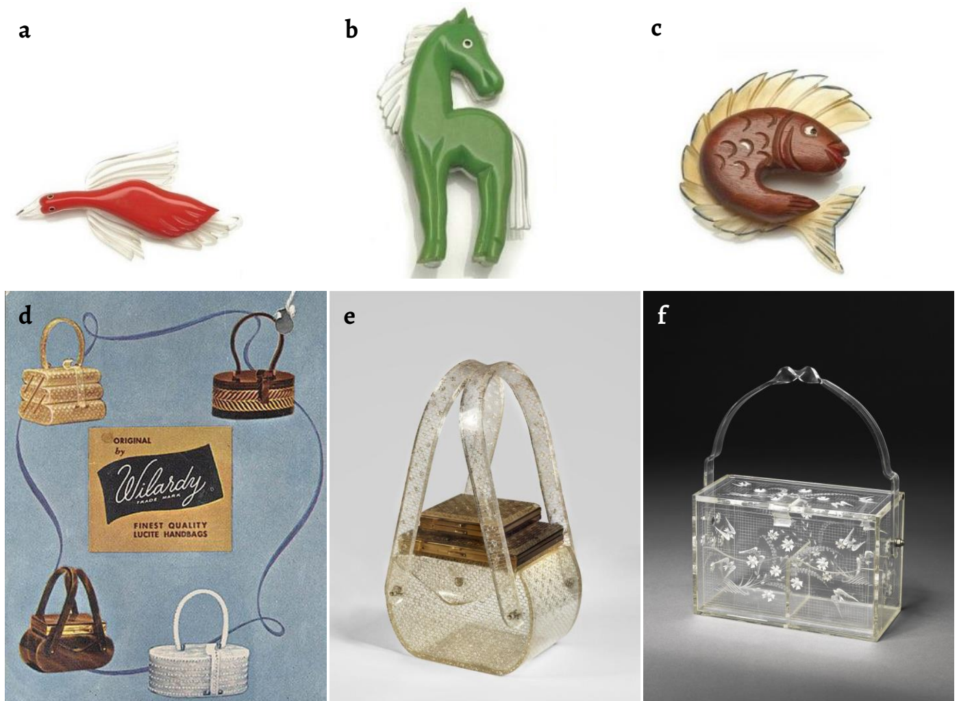
Figure 13. PMMA objects. Plastic jewelry: a) Swan made of Lucite and red Bakelite; b) Green Bakelite and Lucite horse; c) Fish-shaped brooch, Lucite and wood (photo: Leshner, 2005). Bags: d) Wilardy's original advertisement from the 1950s, e) “Stardust” Lucite evening bag, Wilardy Originals, 1950-1960; f) USA Engraved clear Perspex handbag, V & A Museum, London, 2021.
