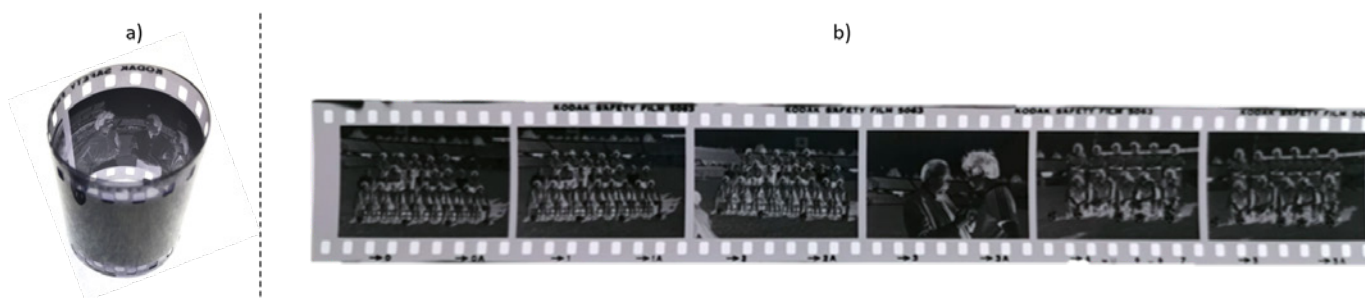
Figure 7. Negative strip: a) before treatment; b) after unrolling and flattening.
