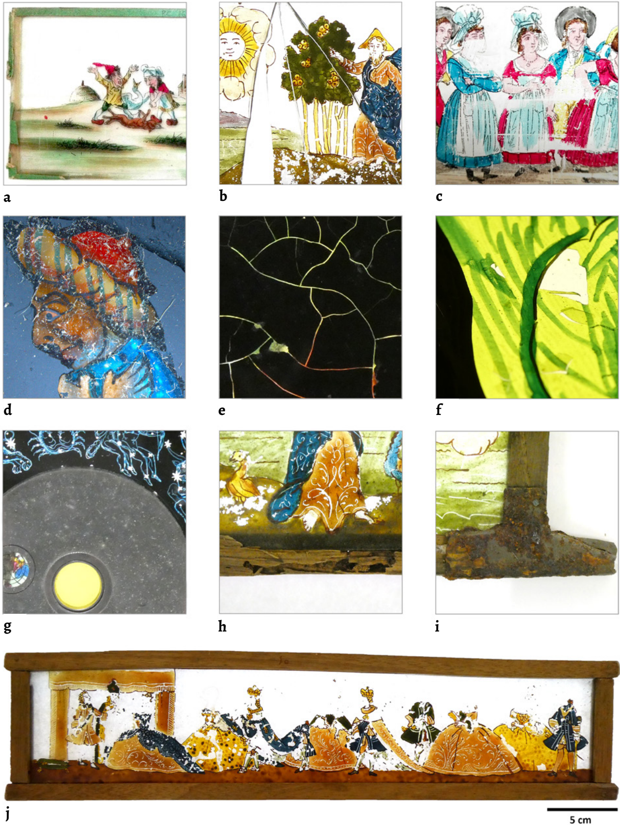
Figure 6. Examples of common degradation problems observed in the slides investigated from CP and MUHNAC collections: a) paper wear and tear (inv. CP_PC165/005); b) glass fracture and lacuna (inv. CP_PC002/011); c) abrasion of the painted surface in preferential direction (inv. CP_PC166/006); d) dust on the surface (inv. ULISBOA-MUHNAC-UL000067); e) cracks pattern on the painting (inv. CP_PC3302/006); f) loss of adhesion and detachment of the paint layer (inv. CP_PC446); g) white spots of deterioration on the enclosed glass surface (inv. CP_PC3301/005); h) wood with insect damage (inv. CP_PC002/011); i) metal corrosion (inv. CP_PC002/011); j) wood distortion (inv. CP_PC002/008) (photo credits CP: Ângela Santos; photo credits MUHNAC: Beatriz Rodrigues).
