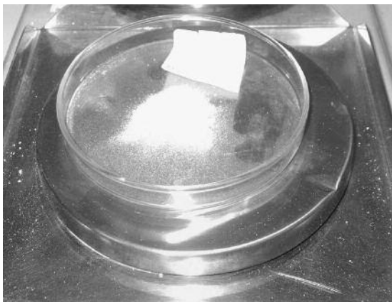
Fig. 1 Residue after drying of the simple limewater.
