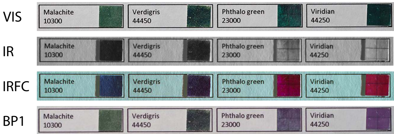
Figure 9. Malachite, verdigris, phthalo green and viridian. Both IRFC and BP1 can differentiate the two historical green pigments (malachite and verdigris) from the modern phthalo green and viridian.
