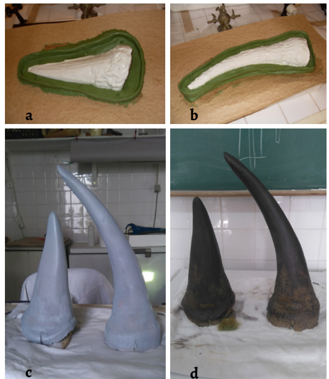
Figure 10. Details of the moulds, support moulds (a-b) and finished horn replicas (c-d) created by Pedro Andrade (MUHNAC).
