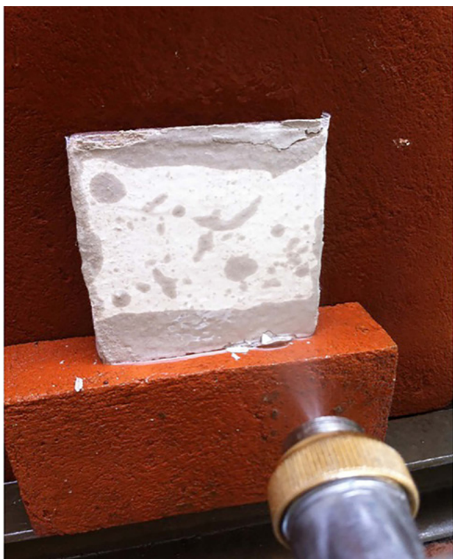
Figure 7. IBAM test sample during the resistance to water abrasion test.
