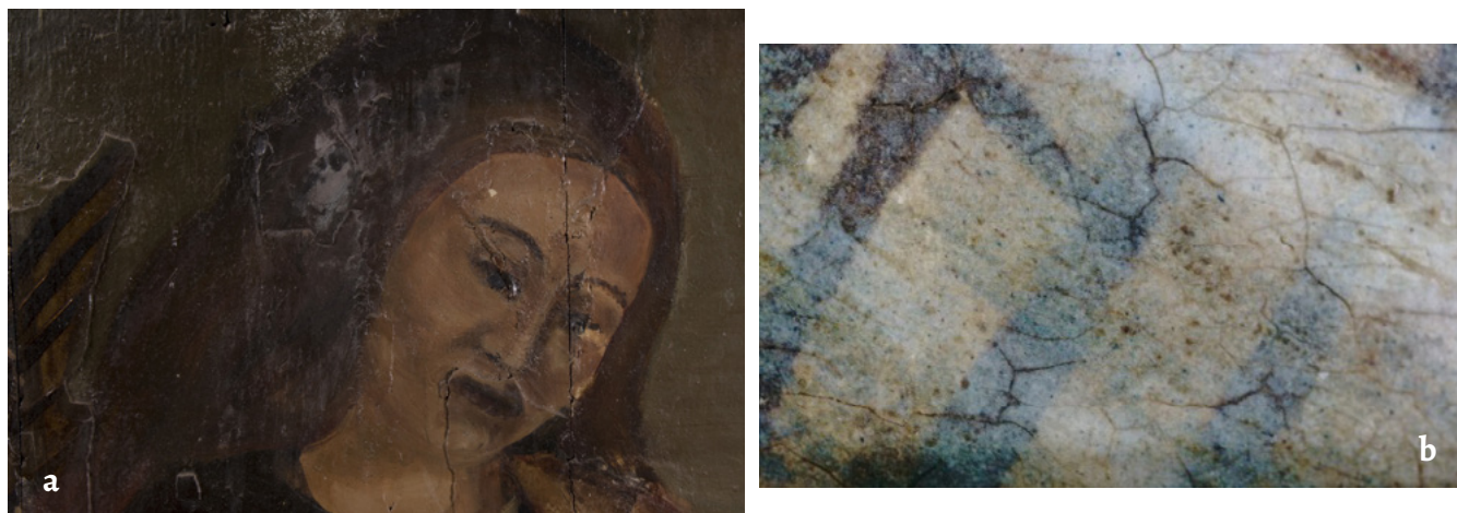
Figure 5. a) Detachment of ground layer from the support causing the flaking of the painting, showing also overpaintings. b) Transparency of painting layers, being possible to see the underdrawings and the ground layer.
