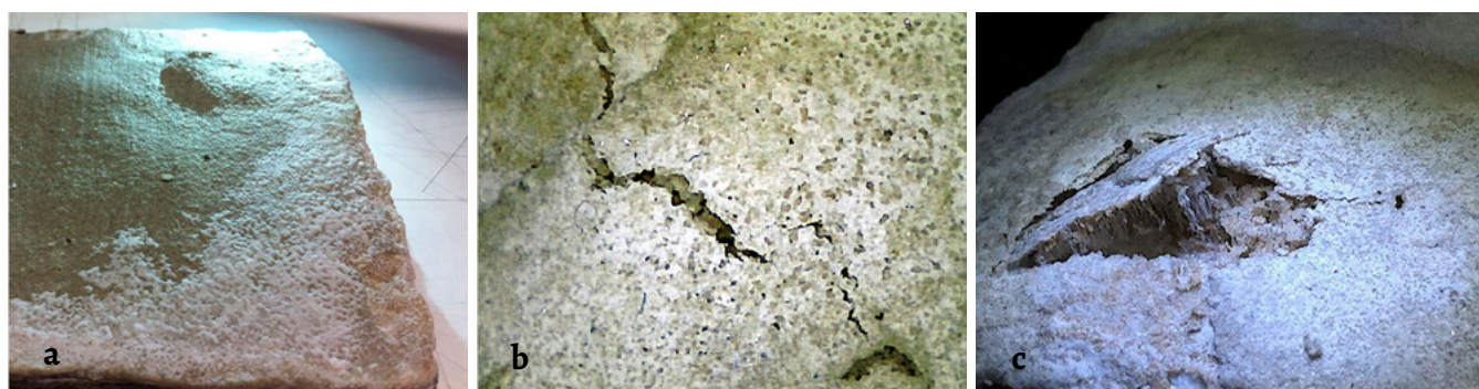
Figure 12. Test sample constituted by a balanced mortar added with nopal mucilage with a layer of clay without interphase mesh (IBA) after the resistance to crystallization of salts test: a) pronounced bulging due to the crystallization of salts on the clay stratum; b) fissures formed on the surface of the sample observed under Aven digital microscope at 20 \times ; c) salt crystals formed in the clay stratum observed under Aven digital microscope at 5 \times .
