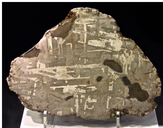
Figure 5. Slice of Nantan iron meteorite showing Widmanstätten figures (weight 3100 g). Museum of Planetary Sciences – Prato, Italy, Inv. No. 1364/2.
