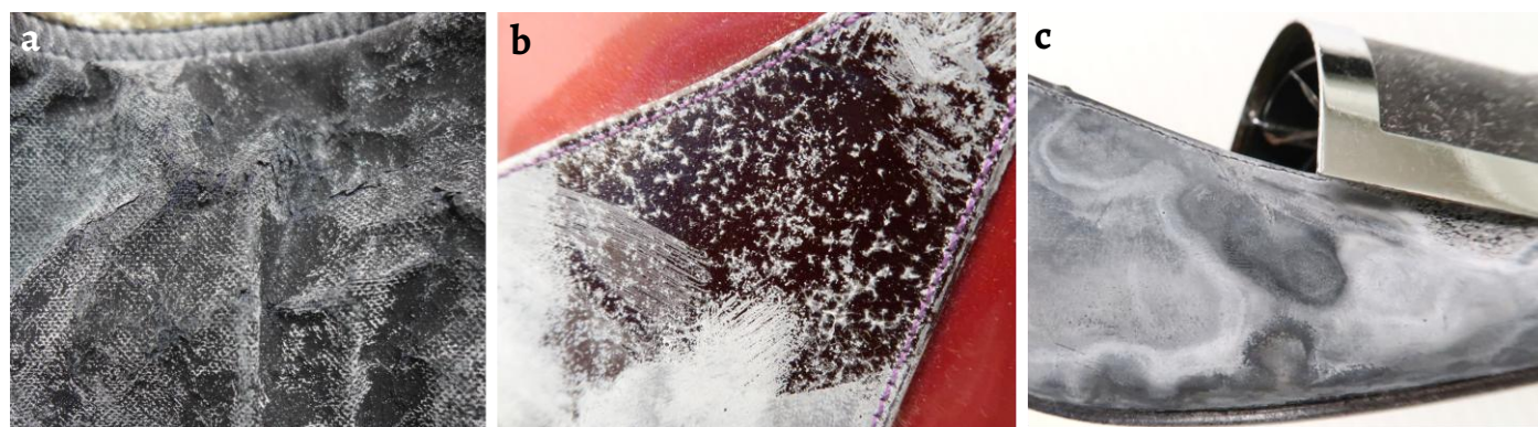
Figure 1. Details of blooming deposits on polyurethane-coated fabrics illustrating different visual manifestations of blooming: a) powder-like deposits; b) dense and dispersed deposits; c) haze-like deposits.
