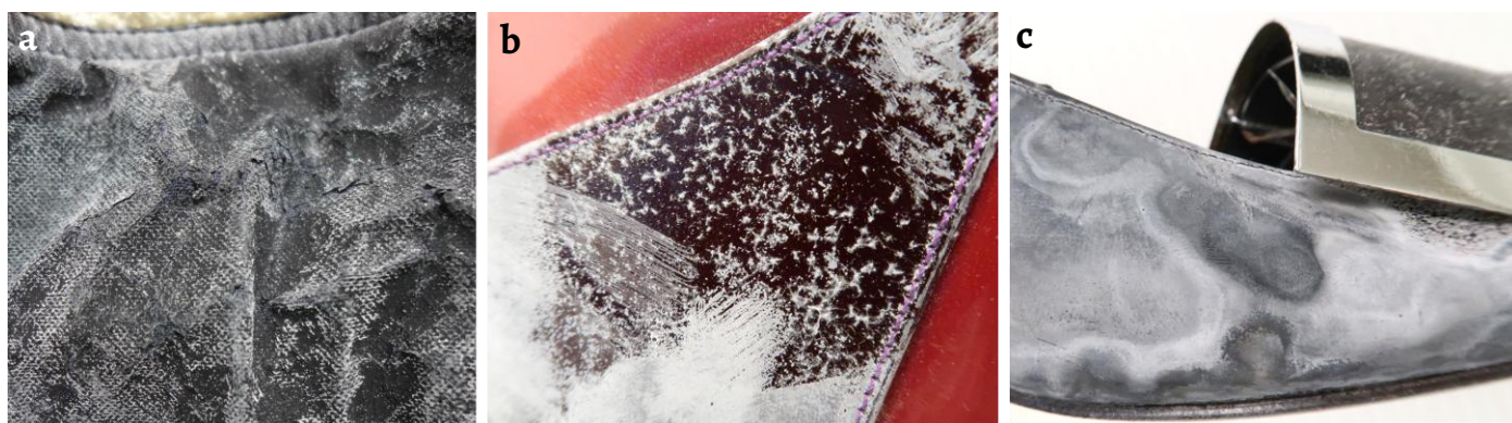
Figure 1. Details of blooming deposits on polyurethane-coated fabrics illustrating different visual manifestations of blooming: a) powder-like deposits; b) dense and dispersed deposits; c) haze-like deposits.
