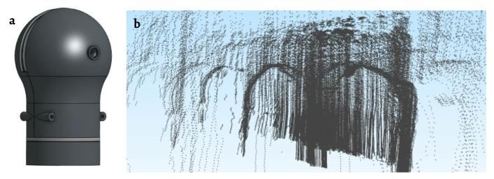
Figure 6. Digitalization of the Mosque Kenadsa Ksar's using laser beam acquisition: a) used LiDAR developed by our team; b) screenshot of the Point-Cloud, Reduced density.
