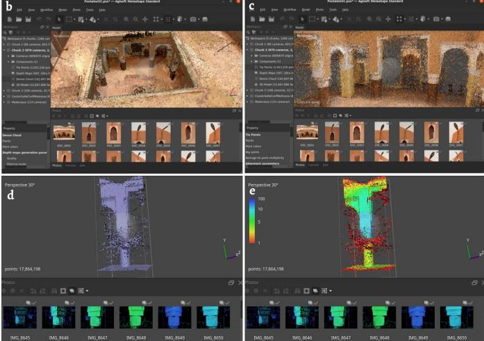
Figure 5. The 3D model of house and column: a) 3D model; b-c) dense 3D point cloud; d) solid model of column; e) Point Cloud and structure confidence.
