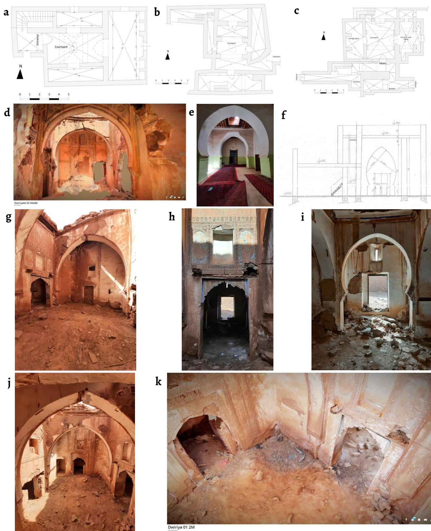
Figure 3. 2D restitution, produced from in situ metric and photographic surveys: a-c) various typology houses; d) 3D model photogrammetry; e) 2D image of courtyard; f) section of old house; g-j) different 2D views of various interior space; k) 3D model in Sketchfab.
