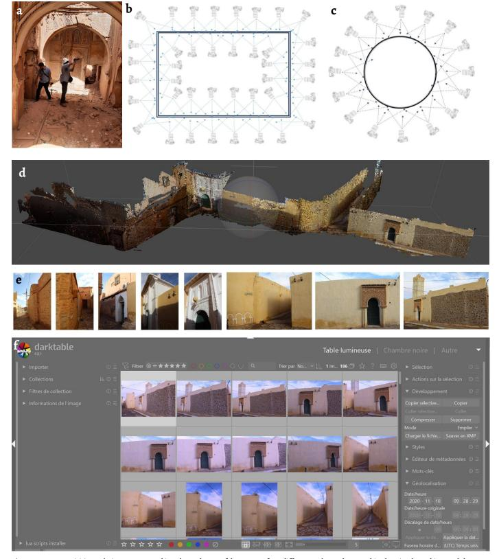
**Figure 4.** Image acquisition techniques: *a*) Team taking photos; *b*) Map of the captures from different angles; *c*) Photographing key circular architectural elements; *d*) 3D Photogrammetry; *e*) a series of 2D images; *f*) Pre-processing.
