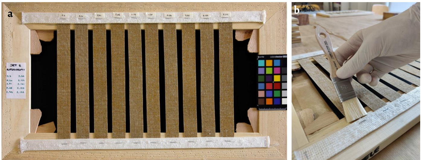
Figure 3. The mock-ups: a) applied on wooden stretchers prior to the application of the consolidants, in order to avoid deformations induced by the use of water-based materials; b) application of CNC.
