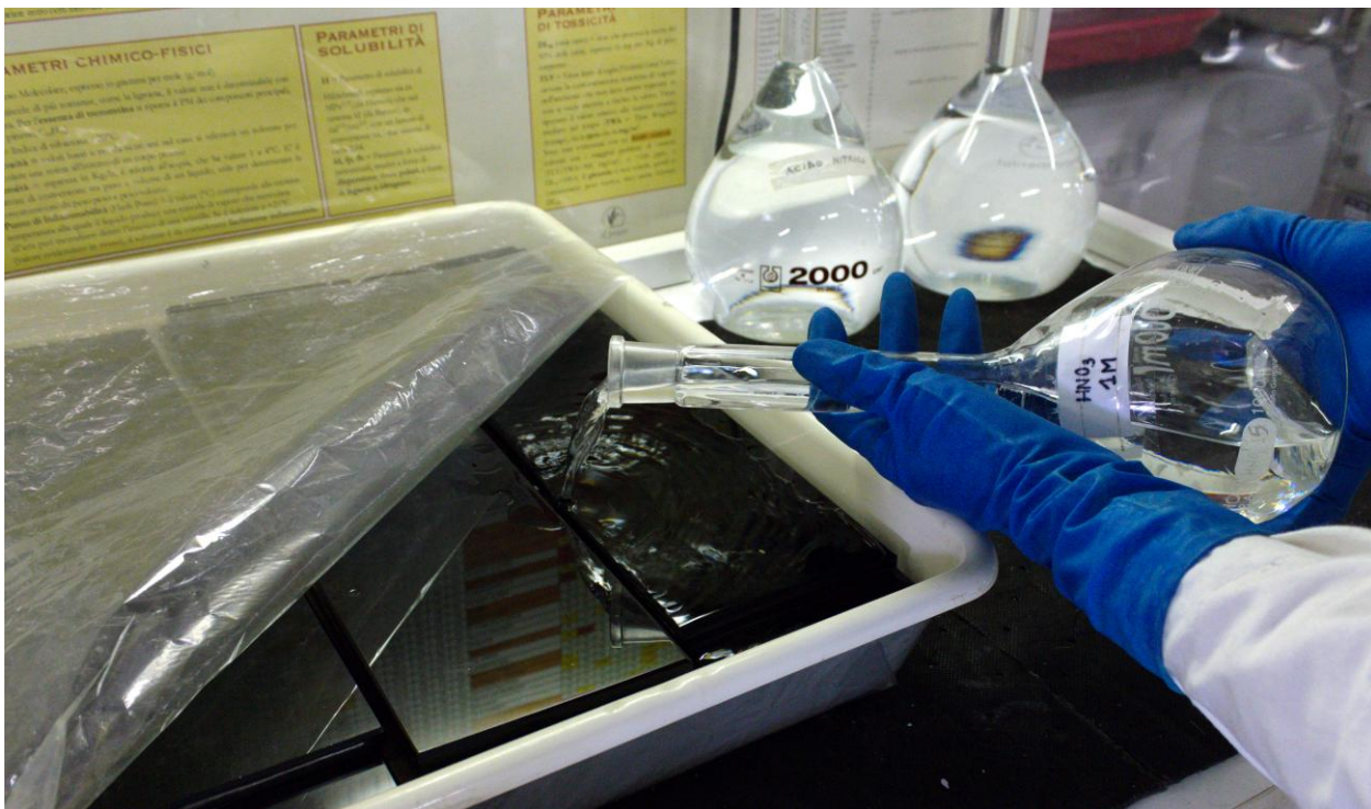
Figure 1. For the depolymerisation of the textile, the linen canvas is put into an acid-resistant box, and glass plates are put on it to reduce its volume. Then, the acid is poured into the box until the canvas is fully submerged. Whereas for this procedure the reference article used a mixture of sulphuric acid and hydrogen peroxide, nitric acid was chosen for this case.
