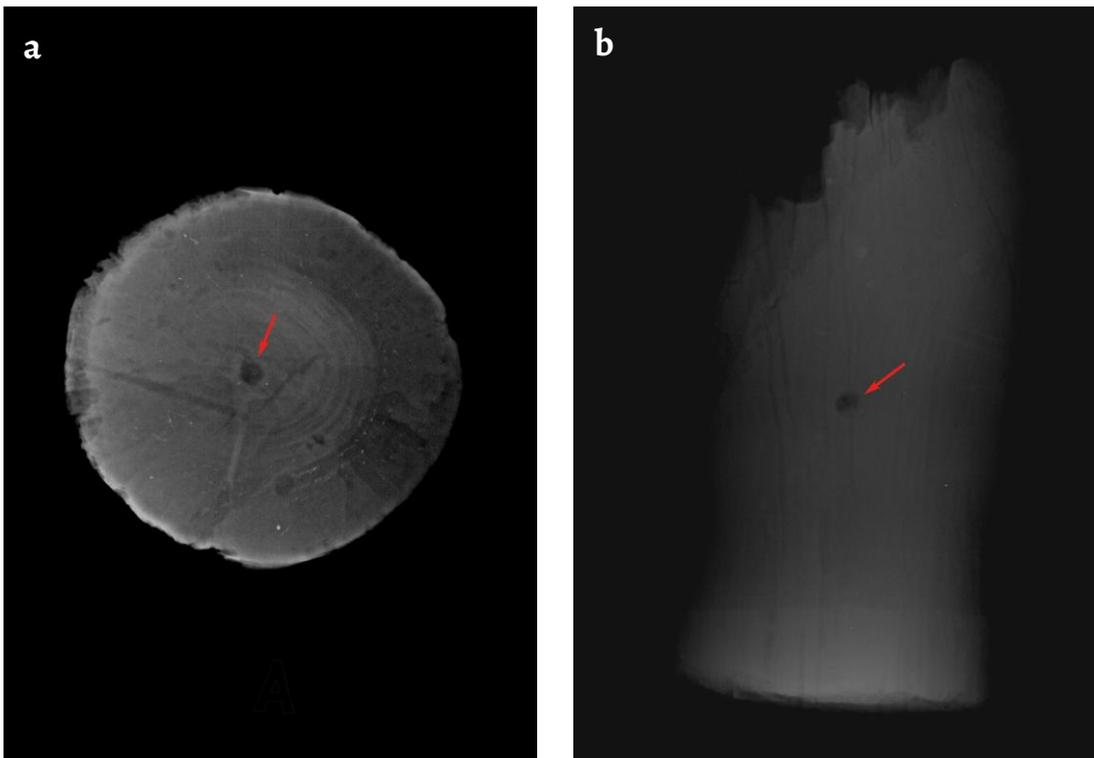
**Figure 3.** X-ray images of samples: *a*) UNT1-A; *b*) UNT1-B. Induced internal damage is visible as the circular shadow in the centre of both samples (photos: J. Harvie and J. Aagaard).
