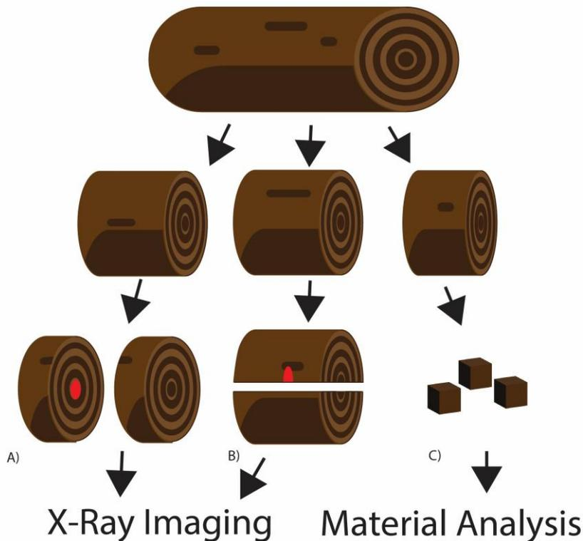
**Figure 2.** Diagram showing the preparation procedure for samples UNT1 and PEG1. Both samples were cut into three sub-samples (A, B, and C). One sub-sample was cut in half across the grain (A), and the other (B) was split in half along the direction of the wood fibre. Red markings show the approximate placements of drilled holes to mimic internal damage. The third sub-sample (C) was used for wood characterisation analysis.
