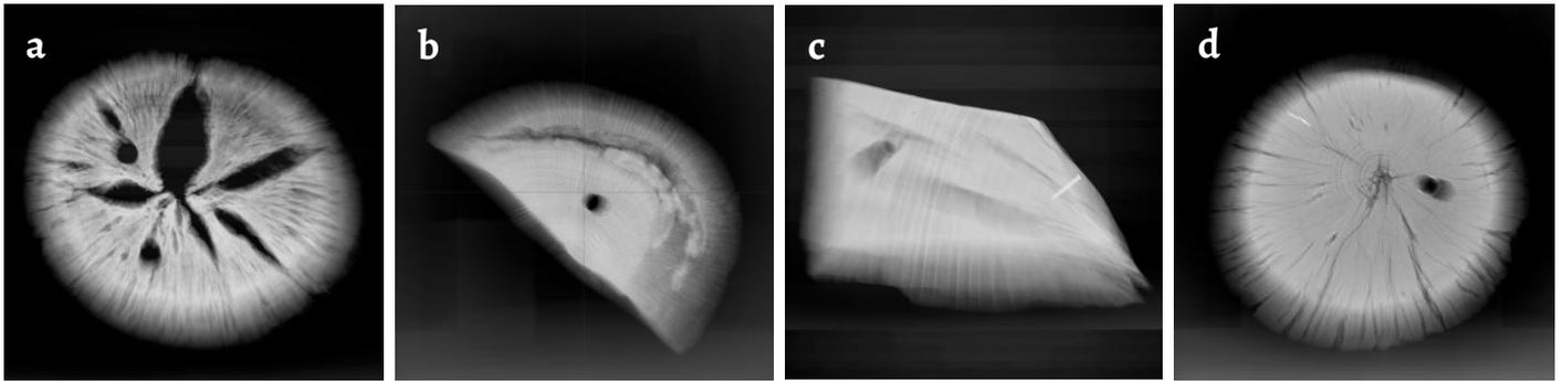
**Figure 7.** X-Ray images of waterlogged archaeological wood samples treated with various conservation agents: *a*) silicone oil; *b*) melamine formaldehyde (Kauramin 800); *c*) lactitol – trehalose; *d*) PEG. Further information on sample treatments is available [19] (photo: J. Stelzner and J. Harvie (RDA)).
