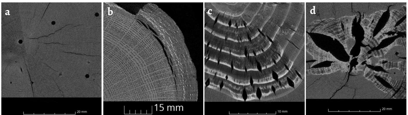
**Figure 1.** Micro-CT images showing the types of internal damage common in treated waterlogged archaeological wood: *a*) radial checking; *b*) ring-shakes; *c*) intra-ring checking; *d*) macroscopic collapse (photos: D. Gwerder – Lucerne University of Applied Sciences and Arts - HSLU, J. Stelzner and J. Harvie)
