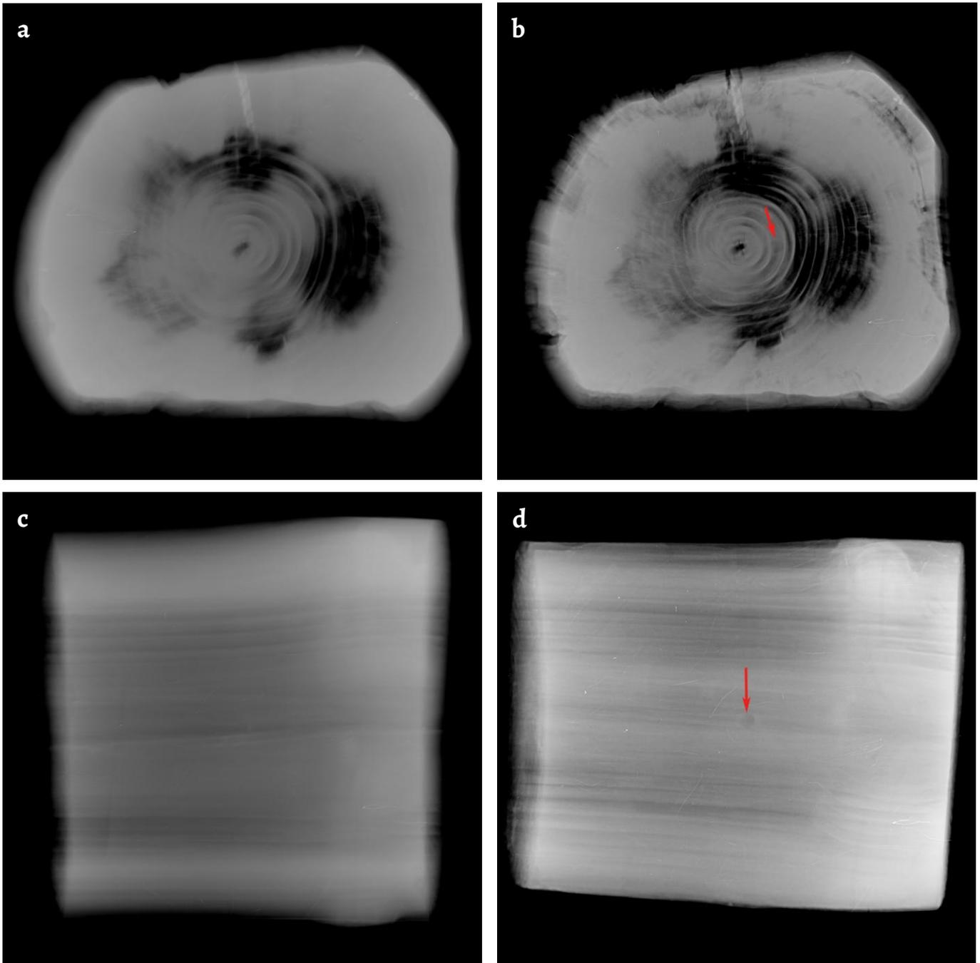
**Figure 4.** X-ray images of wet PEG-impregnated samples: *a)* PEG1-A pre-impregnation; *b)* PEG1-A post-impregnation; *c)* PEG1-B pre-impregnation; *d)* PEG1-B post-impregnation with artificial damage visible in the wood centre as grey shadow (photo: J. Harvie and J. Aagaard).
