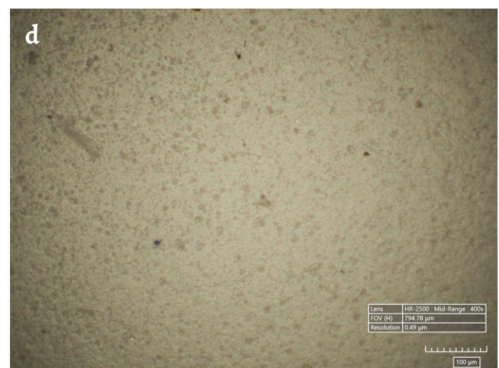
Figure 3. Digital microscopy (Hirox) images showing the surface of Daler-Rowney System 3 Acrylic in: a) lateral and b) coaxial illumination; and Jedynka alkylid enamel in c) lateral and d) coaxial illumination after ageing.
