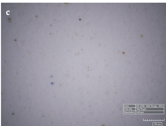
Figure 3. Digital microscopy (Hirox) images showing the surface of Daler-Rowney System 3 Acrylic in: a) lateral and b) coaxial illumination; and Jedynka alkylid enamel in c) lateral and d) coaxial illumination after ageing.
