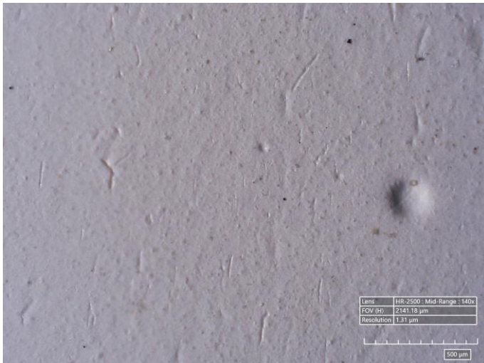
Figure 2. Digital microscopy (Hirox) images showing the surface of Maimeri Polycolor Fine Vinyl Colours in lateral illumination after ageing.
