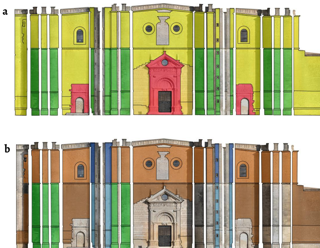
Figure 9. Facade panel analysis: a) materials; b) continuity of bed joints.
