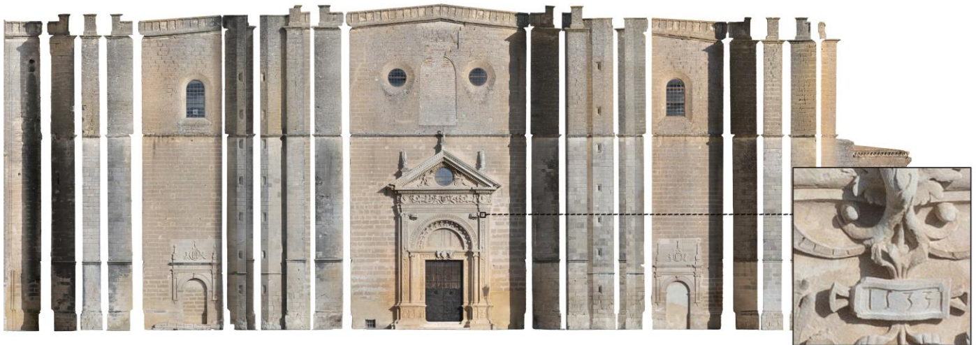
Figure 5. Exploded orthophoto of the main facade and detail of the cartouche from 1533.
