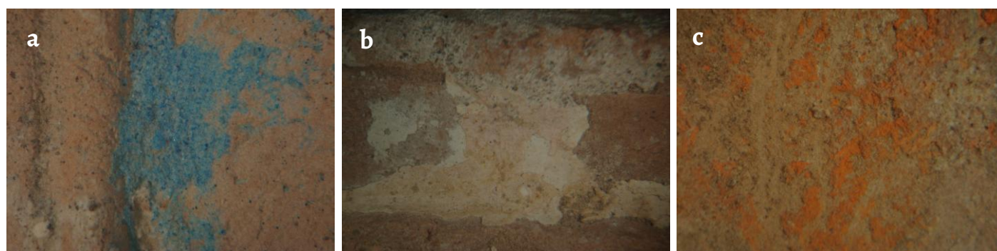
Figure 7. Application of pigments: a-b) blue and orange pigment applied directly on the ceramic surface; c) white pigment applied on the ground (OM).
