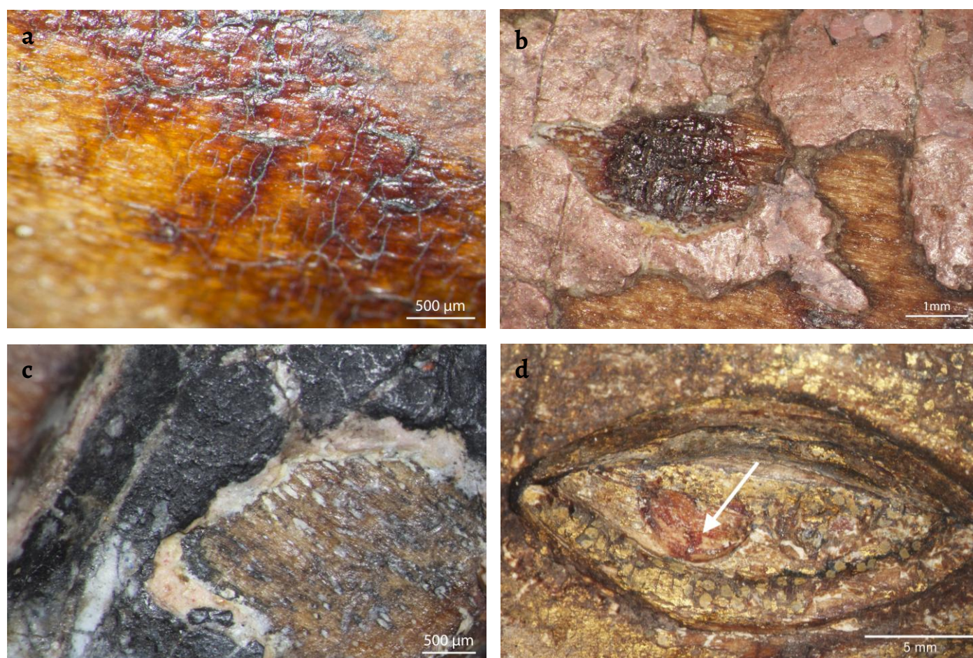
Figure 6. Detail (optical microscopy) of original reddish coating on the dress (a) and face (b), black eye mark (c) and gemstone's red glaze at the cloak's border (d).
