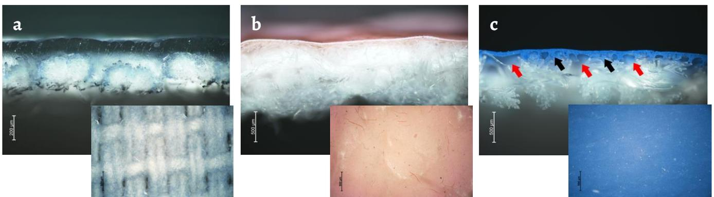
**Figure 3.** Microscopic images of cross-section examples of coated fabrics (see [Table 1](#)) under cross-polarised visible light possibly produced by: *a*) direct method; *b-c*) transfer coating method with complete and partial curing of the coating before lamination of the fabric substrate, respectively (red arrows indicate voids, while black arrows highlight contact areas between the coating and substrate). Insets: top views of the respective coated fabric.
