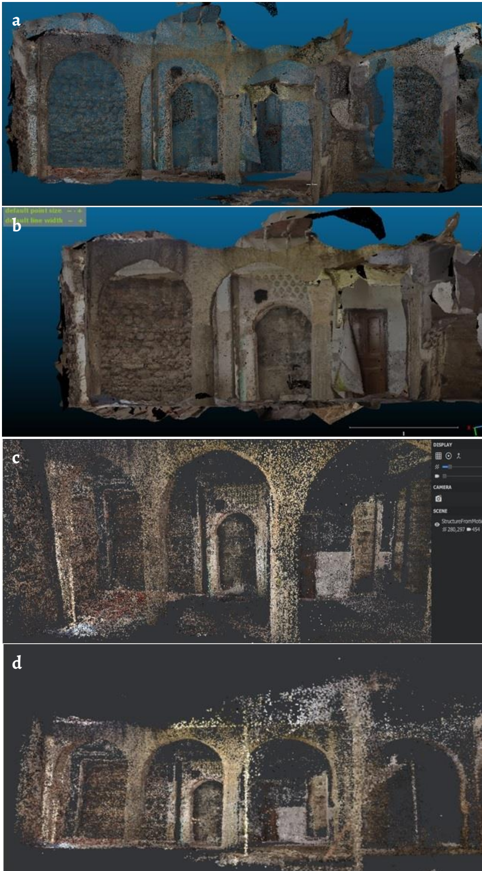
Figure 5. Result of densification points of the prayer room from different angles: a-b ) taken from CloudCompare; c-d ) taken from Meshroom.
