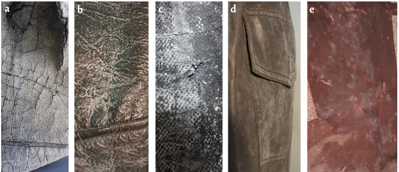
Figure 2. Examples of blooming visual appearance in TPU coated fabrics from fashion case studies produced: a) 1960s; b) 1970s; c) 1980s; d) 1990s; e) 2000s.
