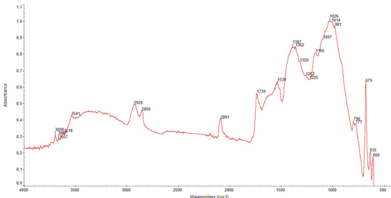
**Figure 17.** FTIR spectrum obtained for bluish colouring area of painting Inv. No. 4082 (Figure 1g).
