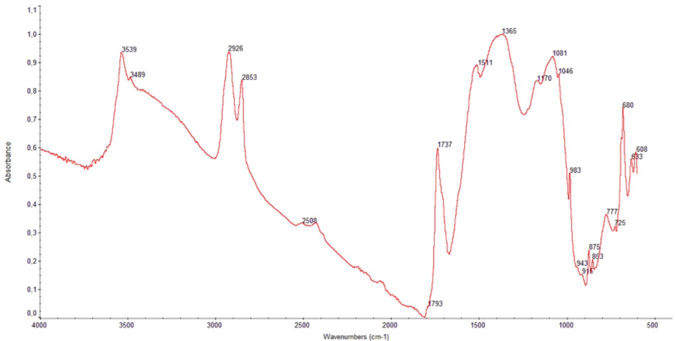
Figure 14. FTIR spectrum obtained for yellow colouring area of painting Inv. No. 4092 (Figure 2bi).
