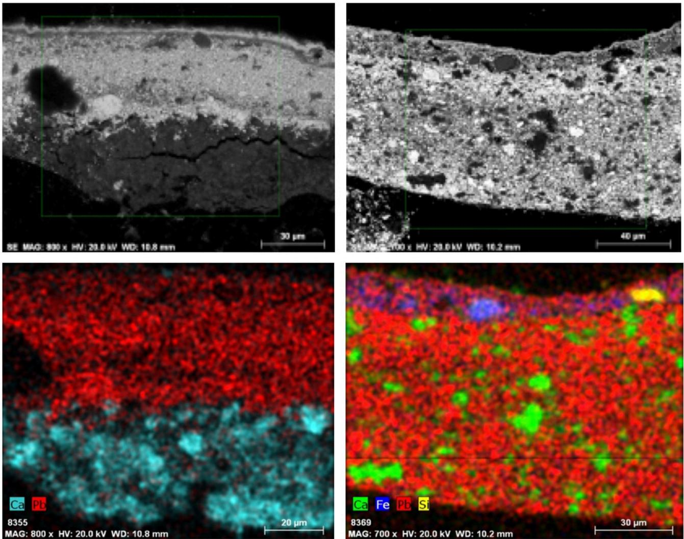
**Figure 9.** SEM-EDS image (a) and (b)) and false colour mapping (c) and d)) of primary layers with Ca (gypsum) e Pb (lead white) of sample 4103-007 (a) and (c) and primary layers of sample 4095-004 (b) and d)) (paintings from Figure 1e and Figure 1i, respectively).
