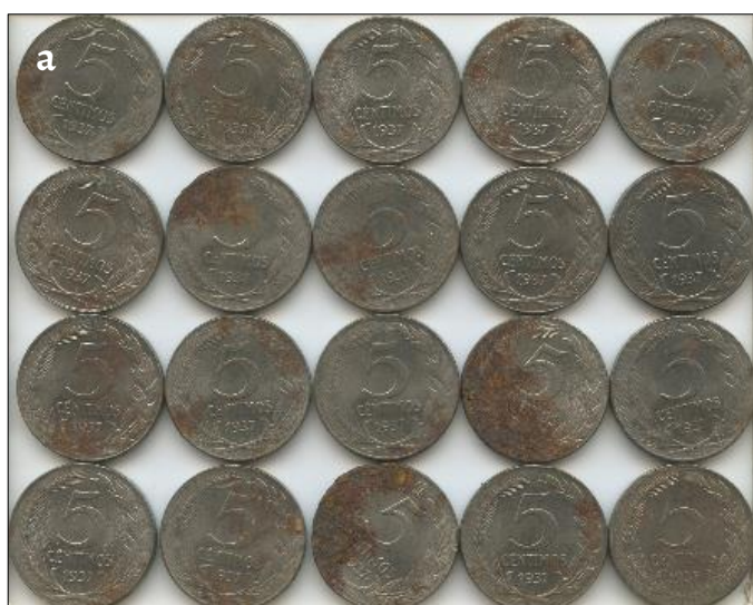
Figure 4. Reverse side of coins sampled from lot 16_1: a) scanned image with tiff format and 31.3 MB size; b) corrosion mapping obtained through Photoshop CS4 software.
